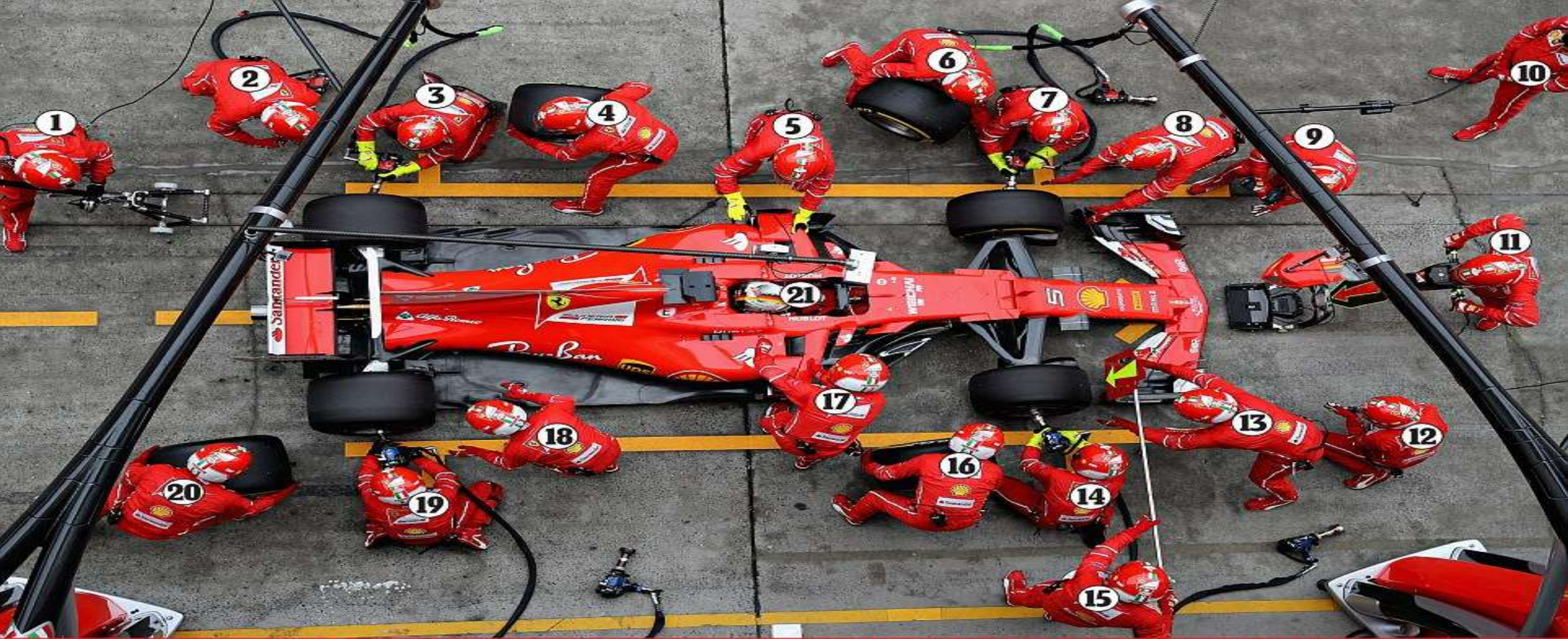
1. Rear Jack 2. Rear Tyre Off 3. Tyre Gunner 4. Rear Tyre On 5. Stabiliser 6. Front Tyre On 7. Tyre Gunner 8. Front Tyre Off/Stop Marker 9. Front Wing Adjuster 10. Backup Front Jack 11. Front Jack 12. Front Wing Adjuster 13. Front Tyre Off / Stop Marker 14. Tyre Gunner 15. Lollipop Man 16. Front Tyre On 17. Stabiliser 18. Rear Tyre Off 19. Tyre Gunner 20. Rear Tyre On 21. Driver
